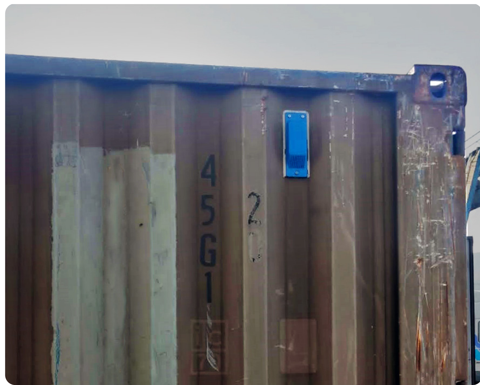
THE HOUSING WITH THE TELEMATICS EQUIPMENT INSIDE, FIXED ON THE WALL OF THE FREIGHT CONTAINER
